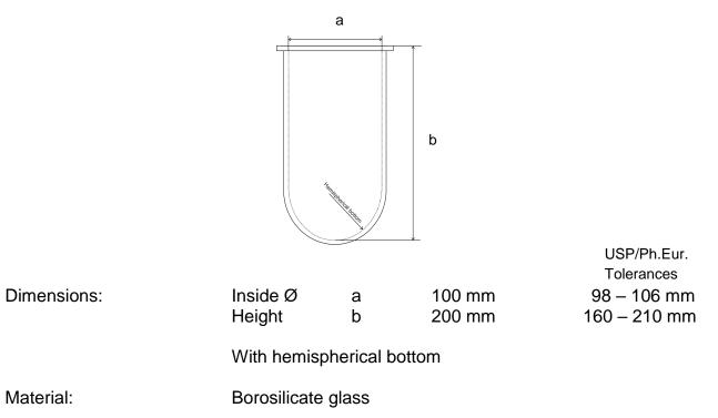
The accuracy of the above mentioned part dimensions have been examined. All relevant measurements are within tolerance and the factory acceptance test has passed. The dimensions are in conformance with USP and Ph. Eur. Pharmacopeia requirements (at time of delivery).
