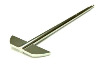
Tolerances Dimensions: Paddle Height 19.0 mm ± 0.5 mm Upper length 74.5 mm ± 0.5 mm Lower length 42.0 mm ± 1.0 mm Size 4.0 mm ± 1.0 mm Radius 1.2 mm ± 0.2 mm Radius 41.5 mm ± 1.0 mm Shaft 9.4 to 10.1 mm Diameter
