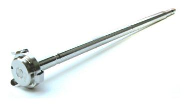
Tolerances Dimensions: Shaft Ø 9.4 to 10.1 mm - -Cap Ø 25.0 mm ± 3.0 mm Cap size 5.1 mm ± 0.5 mm Clear opening 20.2 mm ± 1.0 mm Vent hole Ø 2.0 mm ± 0.5 mm
