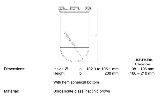
The accuracy of the above mentioned part dimensions have been examined. All relevant measurements are within tolerance and the factory acceptance test has passed. The dimensions are in conformance with USP and Ph. Eur. Pharmacopeia requirements (at time of delivery).
